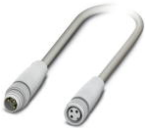
Sensor/Actuator cable, 3-position, PP-EPDM halogen-free, gray RAL 7035, Plug straight M8, on Socket straight M8, Cable length: 3 m, Hygienic design, with plastic knurl
