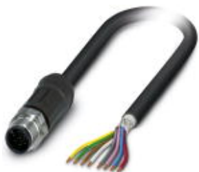
Sensor/Actuator cable, 8-position, PE-X/PE-X halogen-free, black-gray RAL 7021, shielded, Plug straight M12, A-coded, on free cable end, Cable length: 10 m, for outdoor applications, with high-grade steel knurl
