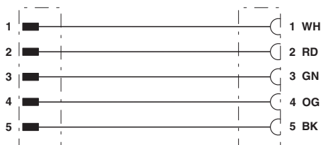
Contact assignment of 7/8" plugs/sockets
