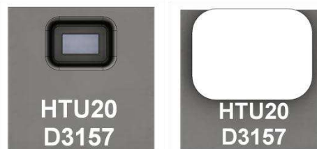
Laser marking on HTU20D(F) sensor
