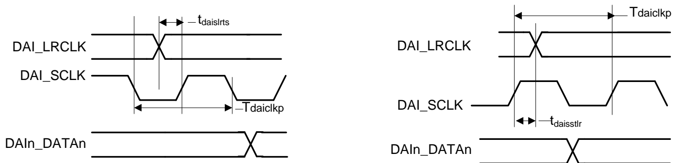
Figure 12. DAI Slave Timing Diagram
