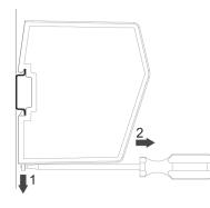
To unmount the device, use a screwdriver to push the DIN-rail fastening mechanism on the back of the device down until it locks in a fixed and open position (1). Then unhook the device from the DIN-rail (2).
