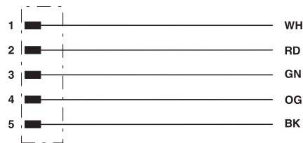
Contact assignment of 7/8" plug
