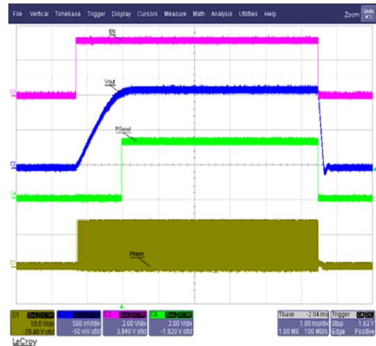
Ch1-Phase Voltage (10V/Div) Ch2-Vout(500mV/Div) Ch3-EN(2V/Div) Ch4-PGood(2V/Div)
