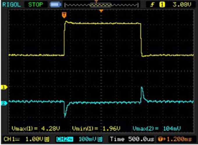
Figure 7. Transient response when load steps from 2A to 4A in PWM MODE.
