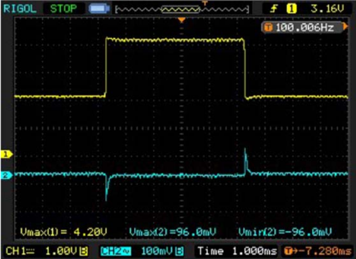
Figure 9. Transient response when load steps from 2A to 4A in PFM MODE.
