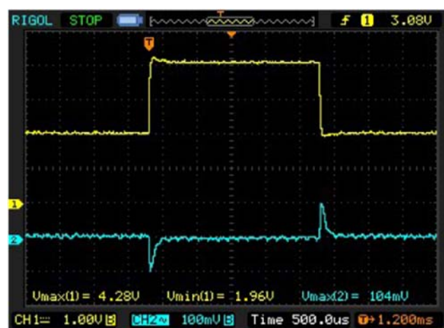
Figure 11. Transient response when load steps from 2A to 4A in DCM MODE.
