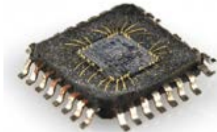
The guts of an integrated circuit, visible after removing the top.
