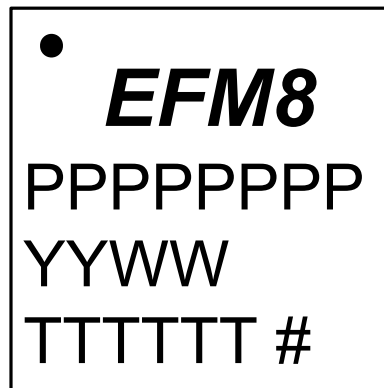
Figure 7.3. QFN32 Package Marking
