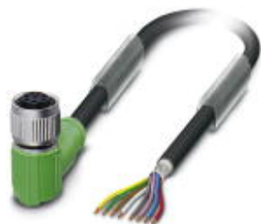
Sensor/actuator cable, 8-position, Variable cable type, shielded, free cable end, on Socket angled M12 SPEEDCON, A-coded, cable length: Free input (0.2 ... 40.0 m)
