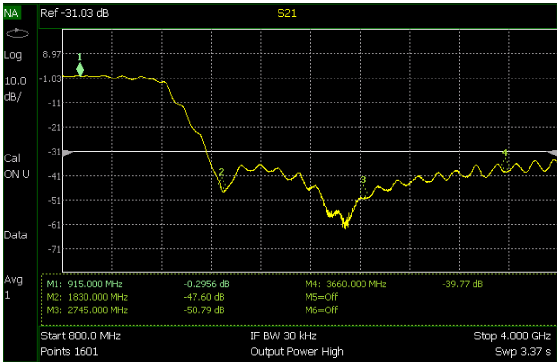
Figure 2 – Ceramic low pass filter characteristic
