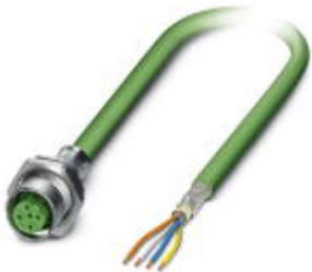
Bus system flush-type socket, PROFINET, 4-pos., M12, shielded, D-coded, SPEEDCON, rear/screw mounting with Pg9 thread, with 2.0 m bus cable, 2 x 2 x 0.34 mm 2
