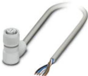
Sensor/Actuator cable, 5-position, PP-EPDM halogen-free, Gray RAL 7035, Free cable end, on Socket angled M12, A-coded, with 3 LEDs, Cable length: 3 m, Hygienic design, with plastic knurl
