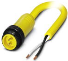
Power cable, 2-position, PVC, yellow, Plug straight 7/8"-16UNF, A - standard, on free cable end, cable length: 1 m
