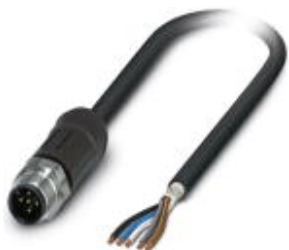
Sensor/Actuator cable, 5-position, PE-X/PE-X halogen-free, black-gray RAL 7021, shielded, Plug straight M12, A-coded, on free cable end, Cable length: 5 m, for outdoor applications, with high-grade steel knurl
