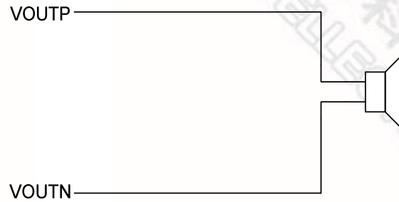
NAU82039 outputs connected to speaker without filter circuit
