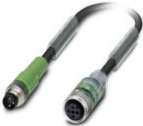
Sensor/actuator cable, 3-position, Variable cable type, Plug straight M8, on Socket straight M12, A-coded, with 2 LEDs, cable length: Free input (0.2 ... 40.0 m)
