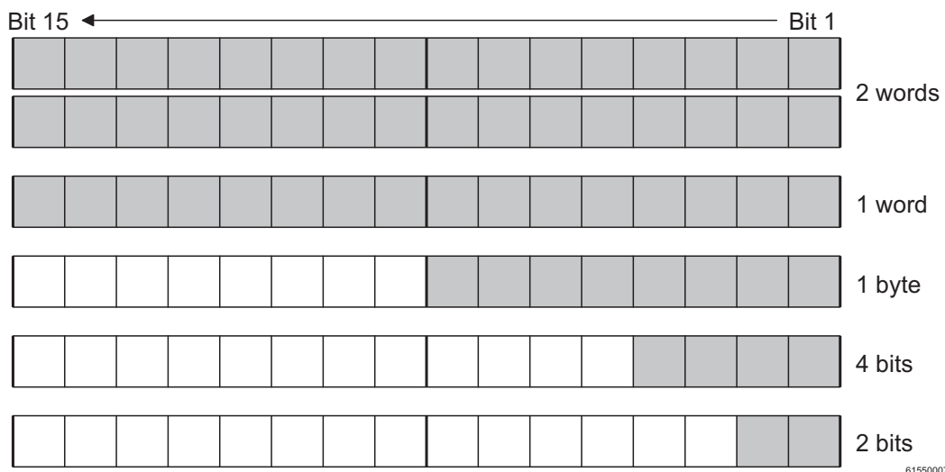
Figure 6 Position of the user data for individual devices in the word array
