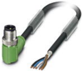
Sensor/actuator cable, 5-position, PUR halogen-free, black-gray RAL 7021, shielded, Plug angled M12, A-coded, on free cable end, cable length: 5 m
