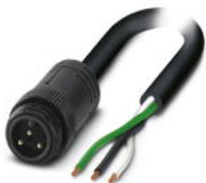
Power cable, 3-position, PVC, black, Plug straight 7/8"-16UNF, A - standard, on free cable end, A - standard, cable length: 5 m
