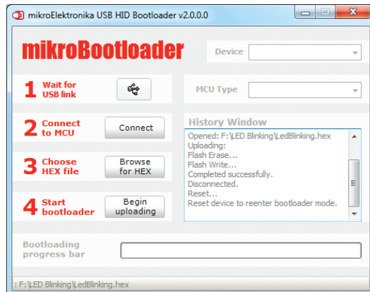
Figure 1-7: mikroBootloader ready for next job
