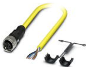
Sensor/Actuator cable, 5-position, PVC, yellow, free cable end, on Socket straight M12 SPEEDCON, A-coded, Cable length: 5 m
