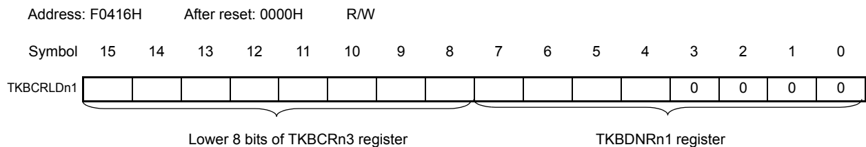
Figure 10 - 15 Format of 16-bit Timer KB Compare 3L & Dithering Count Register n1 (TKBCRLDn1)
