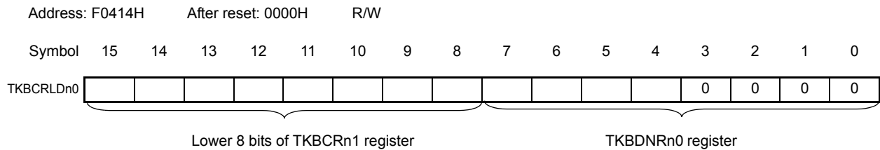
Figure 10 - 14 Format of 16-bit Timer KB Compare 1L & Dithering Count Register n0 (TKBCRLDn0)
